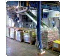
✂ Vacuum lifter to handle effortlessly sacks for an ergonomic working station (option)
