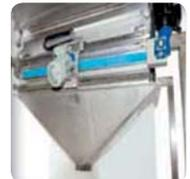
**Vibrating chute** allows to channel the material flow for introduction into the process downstream
