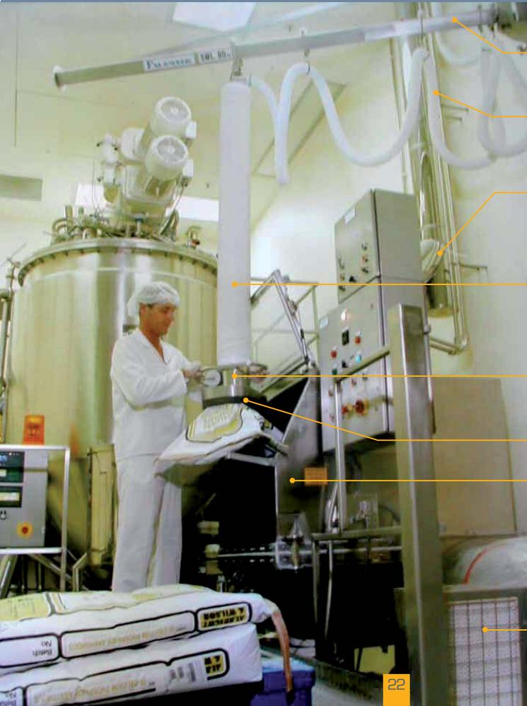
Triangular post mounted jib crane to provide a lifting stroke of 1,700 mm (overhead room 3m.)
