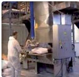
▶ Feeding of the machine with a vacuum sack lifter
