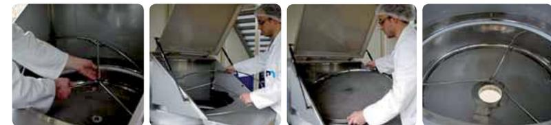
Easy access to the sifter including the screen mesh. Its design allows operators to clean and replace the screen mesh in seconds.
