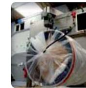
➤ **Screw compactor** for the evacuation of the emptied sacks and the reduction of dust emissions
