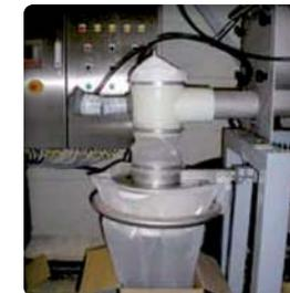
Conditioning unit at the output of a though screw conveyor
