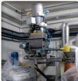
Cyclone transfer system with dosing device
