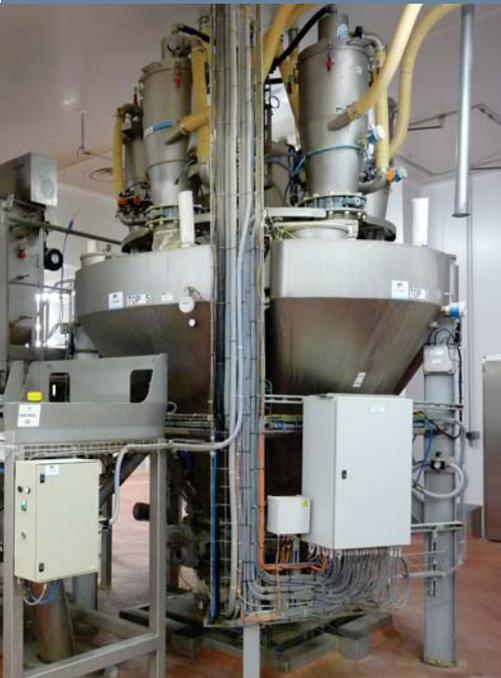
The vacuum dense phase conveying technology allows the integration of weighing solutions.
