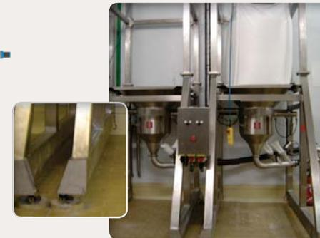
The loss-in-weight of the starting points combined with line purging provides complete dosing for conducting the premix.
