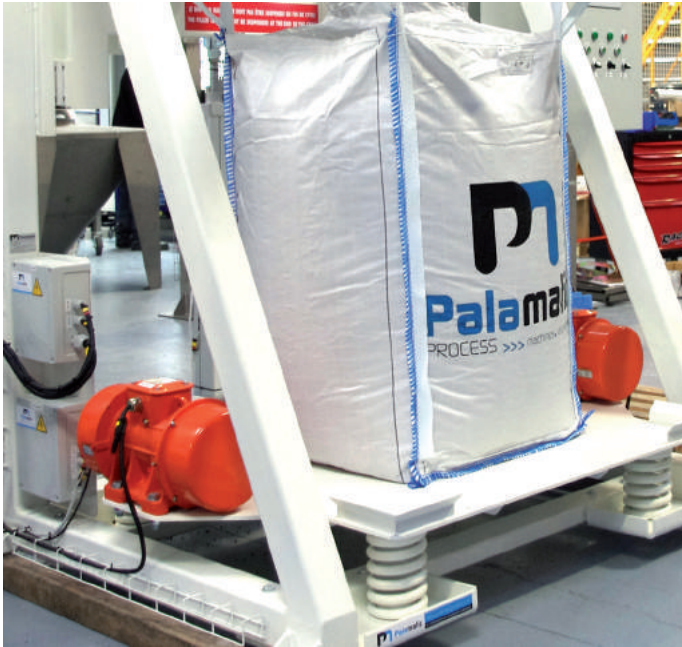
Vibrating table to ensure product densification to obtain a stable big bag
