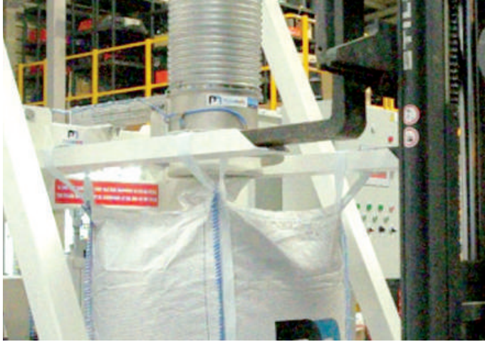
«U» shaped forks for removal of the bulk bag by the handles without the use of a pallet
