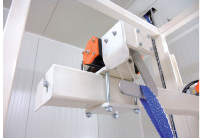
Automatic release of the handles for ergonomics and high rates
