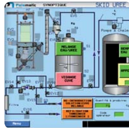
Control of a urea skid
