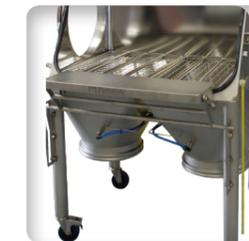
▶ **Product outlet chute adapted to each particular case:** the slope of the hopper allows clearance for knees and feet
