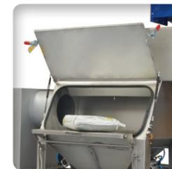
▶ **Access door mounted on gas spring:** an accompaniment to the opening and closing
