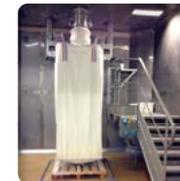
▶ **Suspended structure:** facilitates floor cleaning
