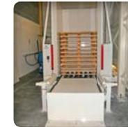
Pallet unloader can handle 15 multistyle pallets
