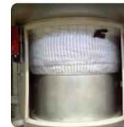
▶ **Anti-overflow tube:** to ensure the containment of product flow during the big bag cuff opening phase and to offer more ergonomics and safety to the operator
