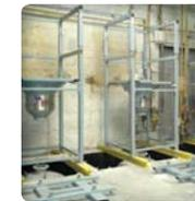
▶ **Frame adjustment of the station:** height adjustment by a manual system of rods. Thus, big bags with any dimensions are admissible on the station
