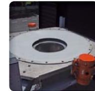
▶ **Containment:** the rubber seal optimizes containment by capping the bottom of the big bag and enables to channel the air flow from dust collector
