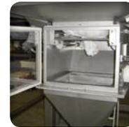
▶ **Control valve:** this flow regulation system works through two pneumatic cylinders. The operator can stop or regulate the flow of the powder
