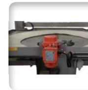
▶ **Pulsed vibration:** if the material requires further inducement to achieve a steady flood feed state at its outlet, an electromechanical (or pneumatic) vibrator mounted to the hopper provides additional flow inducement
