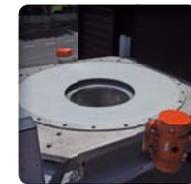
▶ **Rubber seal:** to optimize the containment during the emptying phase (optional)
