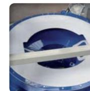
▶ **Connection to the dedusting unit (optional):** the dedusting ring is mounted on the receiver plate and minimizes dust emissions. It is composed by a split tube and a pipe for connection to the dedusting unit. It is manually operated to adjust or close off the suction flow
