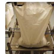
▶ **Improvement of bulk material flow (optional):** the bulk material flow is optimized thanks to a pneumatic massager system. Pneumatic cylinders are implanted on the lower part of the structure, crush severely agglomerated lump into smaller chunks (2, 4 or 6 actuators depending on the type of powder)
