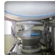
➤ **Total dust containment with tensioning and docking cylinder:** it provides a dust-tight seal with the discharge spout of the big bag and eliminates the potential for contaminants to enter the process. The pneumatic cylinder enables the operator to adjust the connection height to fit different big bag sizes
