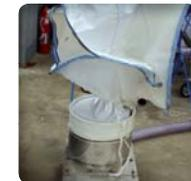
➤ **Putting big bag under vacuum (optional):** at the end of emptying process, the operator can put the big bag under vacuum using dust collector to avoid dust emanation into production facilities
