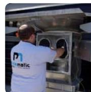
▶ **Containment and operator protection:** the glove box with a dust-proof door provides a secure and ergonomic access to the big bag spout. The respect of the sight height allows the operator to manipulate big bag without being in contact with potential toxic materials
